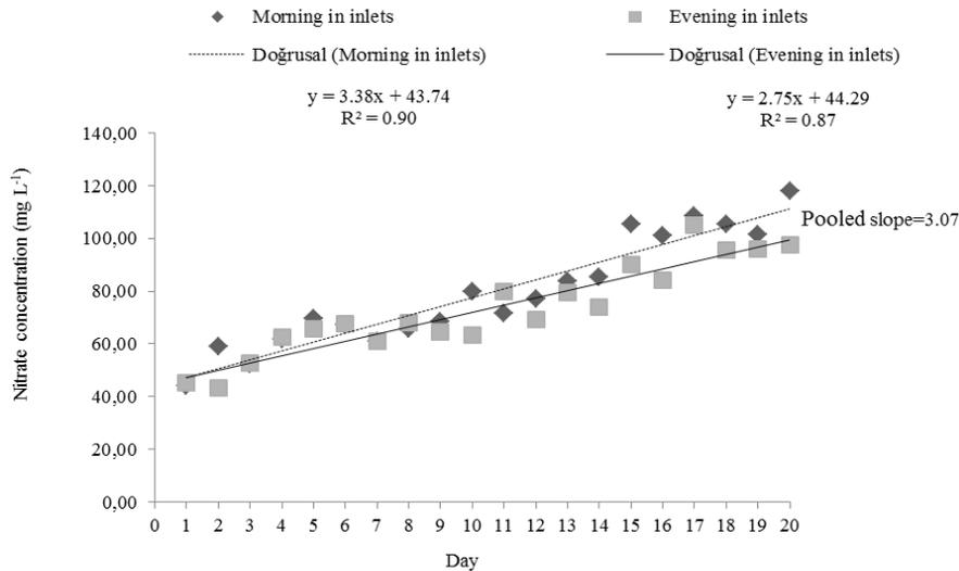
**Figure 3.** Nitrate (NO<sub>3</sub><sup>-</sup>) concentration at the inlet in the morning (07:00h) and in the evening (18.00h) during the experiment.
