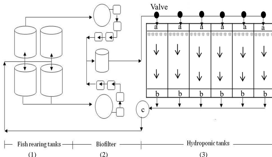
**Figure 1.** Schematic representation of the ARDA aquaponic system consisting of 3 components. (1) = Four fish rearing tanks (2) = Biofilter; one biofilter tank, two solid removal tanks, eight filter tanks with nets (3) = Hydroponic tanks; in this experiment, six hydroponic tanks were used a = Water inlet and sampling point b = Water outlet and sampling point c = Sump ● = Valve.
