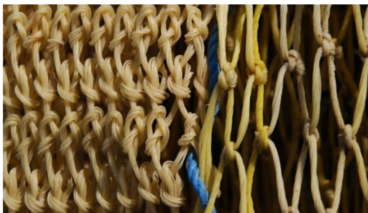
Figure 2. Hand-woven (left) and machine-woven (right) codends.
