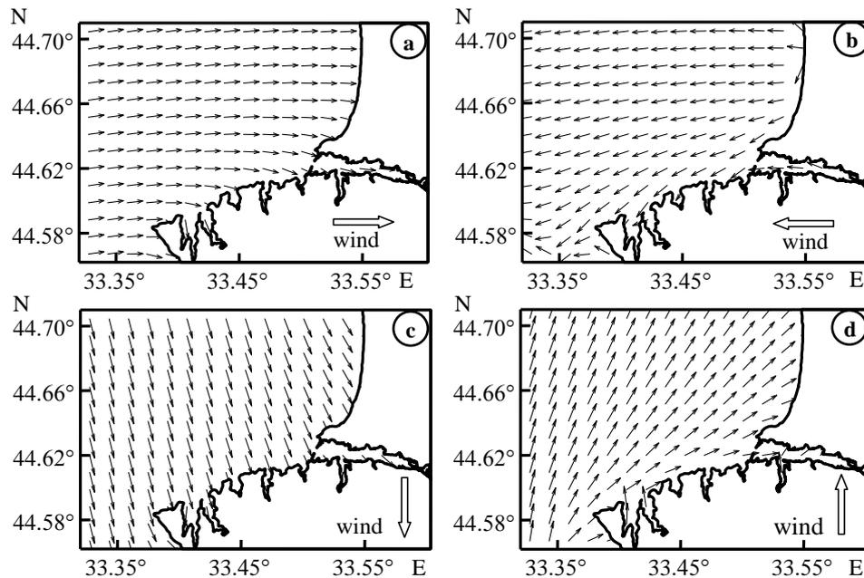
**Figure 4.** Wave direction near the south-west coast of the Crimea in case of west (a), east (b), north (c) and south (d) winds.
