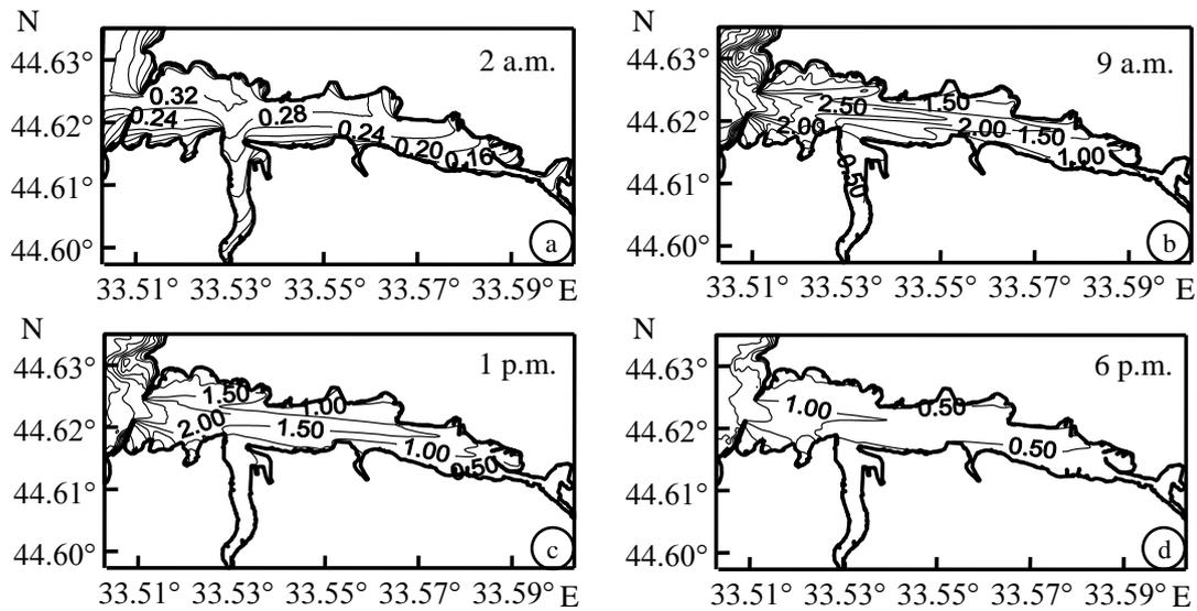
**Figure 5.** Significant wave heights (m) in the Sevastopol Bay on 11 November 2007 at 2 a.m. (a), at 9 a.m. (b), at 1 p.m. (c) and at 6 p.m. (d).
