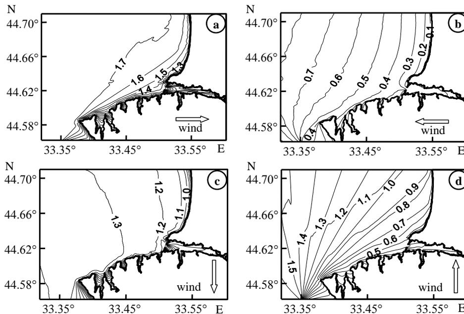
**Figure 3.** Significant wave heights (m) near the south-west coast of the Crimea in case of west (a), east (b), north (c) and south (d) winds.
