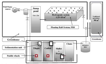
Figure 2. Schematic diagram of the IMTA-FRS.
