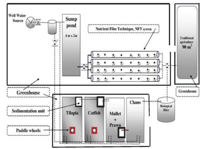
Figure 3. Schematic diagram of the IMTA-NFT.
