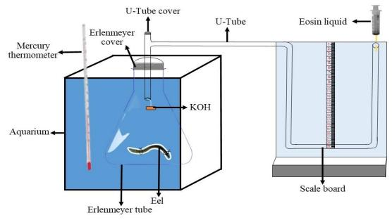
Figure 1. Volumetric respirometer design
