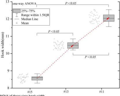
Figure S2. One-way ANOVA of three sizes hook width
