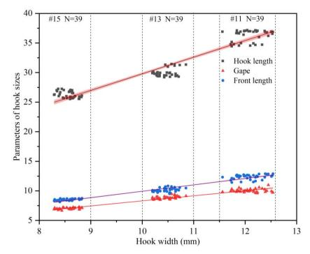
Figure S1. Relationship between parameters of hooks
