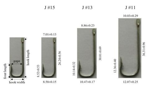
Figure 2. Shape and dimensions of three size hooks used in the selectivity study. Means and standard errors based on a sample size of 39 hooks for each type.
