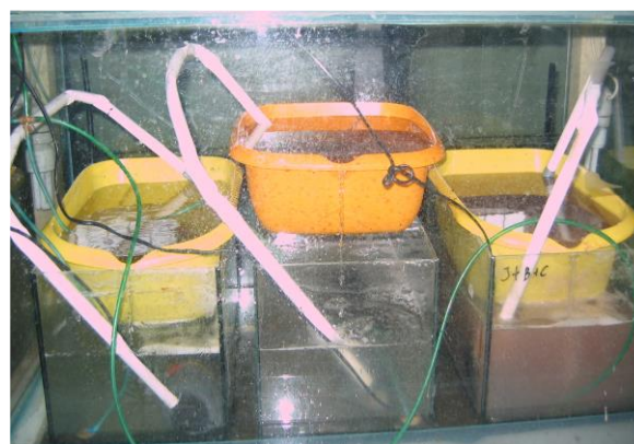
Figure 2. Three plastic container sets of worms in only-water exposure. The container with the worms is in slight inclination of 8% in order to have drop in water levels. Water is circulating through the pump located in the aquarium under the container.
