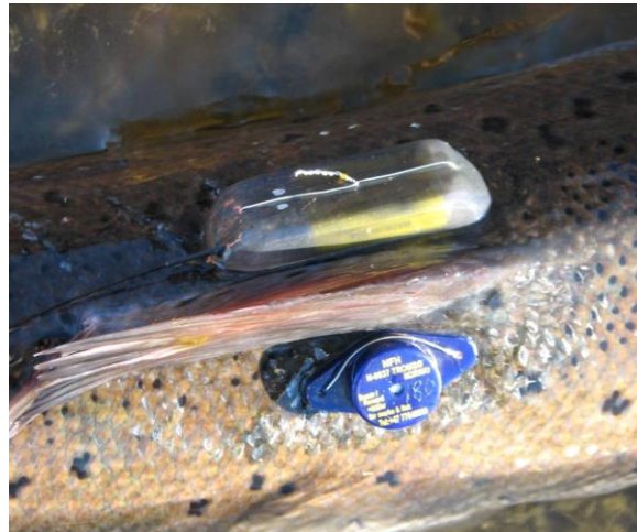
Figure 6. External attachment with a radio transmitter on one side and a data storage tag (DST) on the other side of the dorsal fin. Such double tagging is only suitable for large fish. Photo: Audun H. Rikardsen.
