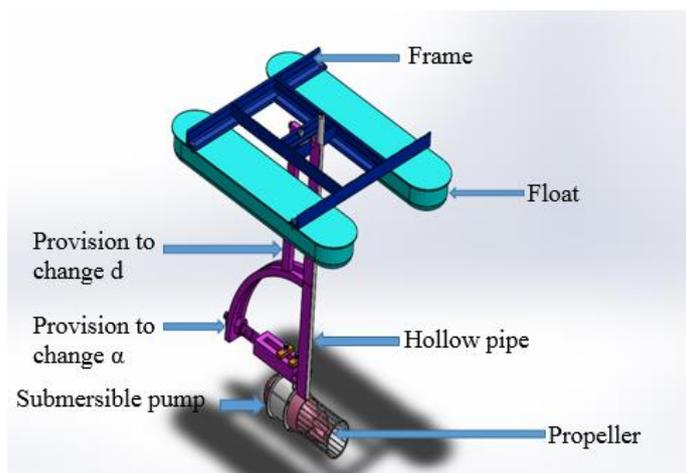
**Figure 2.** A view of submersible aerator after modification.
