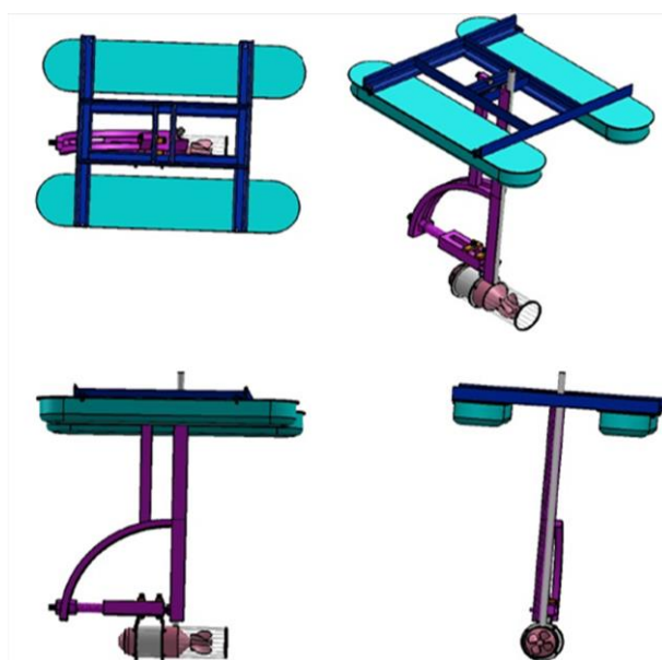
Figure 3. Different views of the modified aerator.
