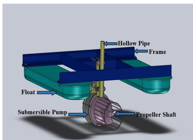
**Figure 1.** A view of submersible aerator before modification.**Table 2.** Specifications of the aerator
