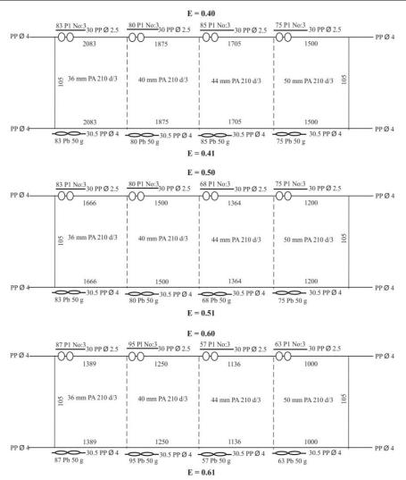
Figure 2. Connected nets (E = 0.40, 0.50, 0.60) with different hanging ratio.
