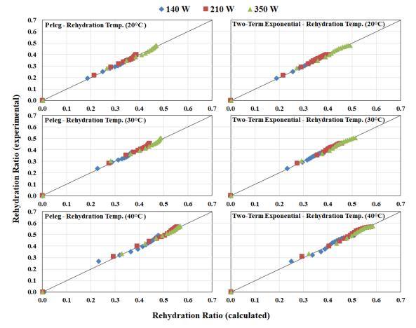
Figure 6. Experimental and calculated rehydration ratio values of Peleg and Two-Term Exponential models.
