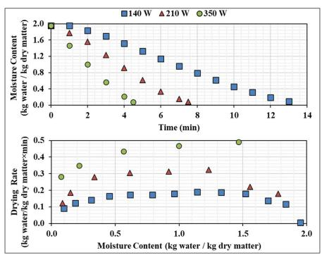
Figure 1. Drying curves of mussels at various MW power levels.
